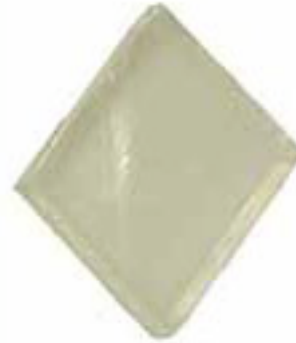
The mineral calcite has three cleaving planes. The result is a shape called rhombohedron.
